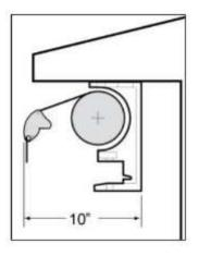
**WARNING!** Proper positioning of the supports is the most important and critical step in erecting the awning. It is imperative that all screws are well anchored to the rafters or other major structural elements.
