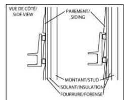
**WARNING!** There are often furring strips on top of the fibreboard, wider than the stud. The lag bolt must be installed in the stud, not just in the piece of wood and not just in the furring strip. Probe the chosen spot with a small drill bit before installing, to avoid shattering the stud by drilling too close to its edge.
