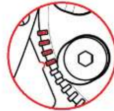
Screw (1,3) visual adjusting guide
